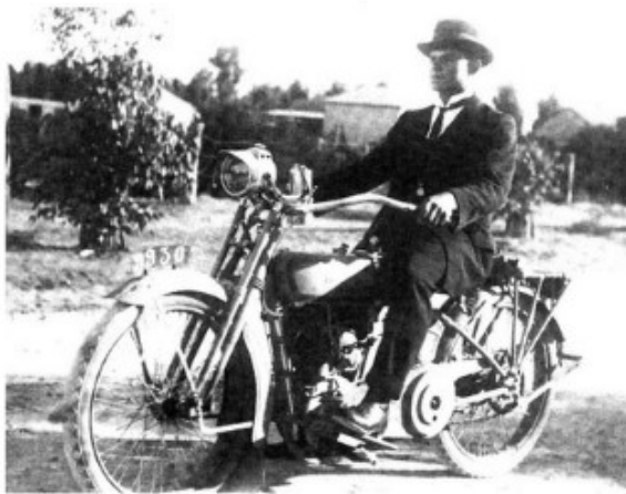
Harley Davidson 500 cc single c.1918. Most were twins, but the Bosch magneto can be seen where the second cylinder would be. Johannes Lange, Tanunda
