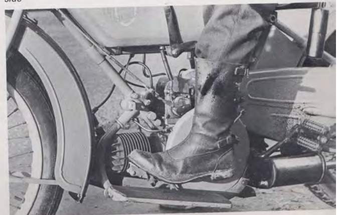
(Above) The John-Manville speedometer, reading to 80 mph, has both total and trip recorders. The 3-speed gearchange quadrant labels middle as second and top as high. (Below) The outside flywheel is shielded by a pressed-steel cover but nothing seems to have shielded the rider's boot from annointment with the GTX. This rocking pedal controls the foot clutch. Brake is on the carburettor side
