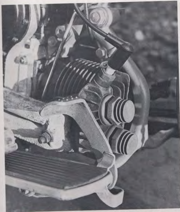
Footboards and forward controls are featured. Fircone caps are situated in the usual way over the side valves. Plugs are of course 18-mm. Note the radial finning to the cast-iron head. Pistons are also ferrous
