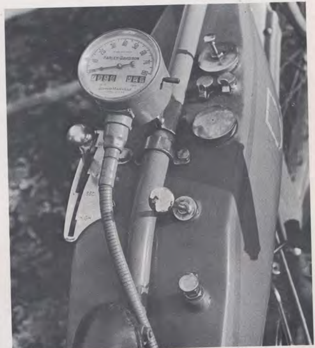
(Above) The John-Manville speedometer, reading to 80 mph, has both total and trip recorders. The 3-speed gearchange quadrant labels middle as second and top as high. (Below) The outside flywheel is shielded by a pressed-steel cover but nothing seems to have shielded the rider's boot from annointment with the GTX. This rocking pedal controls the foot clutch. Brake is on the carburettor side
