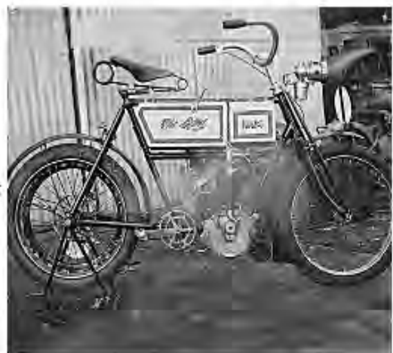
This Lewis was number 6 of Lewis' production. It was a watercooled Blumfield engine.
