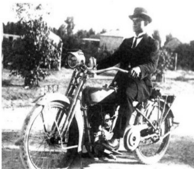
Harley Davidson 500 cc single c.1918. Most were twins, but the Bosch magneto can be seen where the second cylinder would be. Johannes Lange, Tanunda
