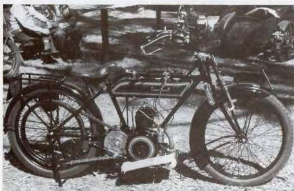
96. Sparkbrook. A little known English make. This 1923 was brought out from the U.K. by Brian Farmer in recent years and has been rallied extensively. 269c.c. Villiers Motor. Eng/No. JB1, F/No. 3126 C.
