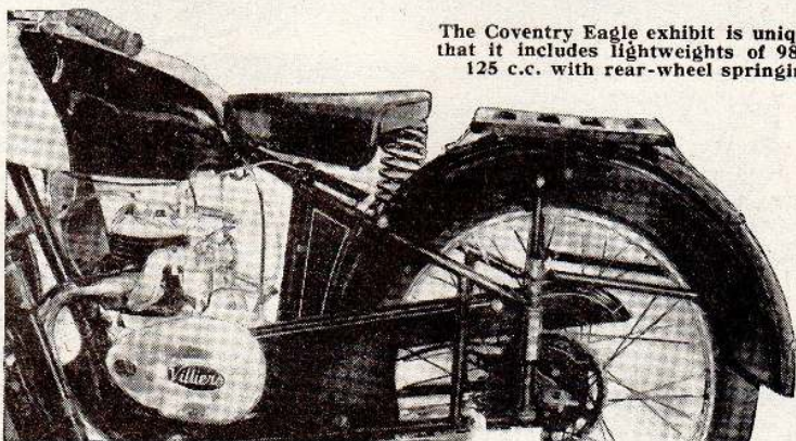
Simple construction of the spring frame that is fitted to the machine illustrated below
