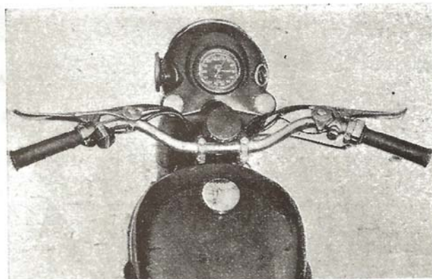
Rider's view of the new headlamp cowl; light switch is on the left, ammeter on the right
