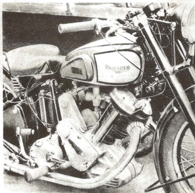
Using the engine to form part of the frame has been a feature of the Model 100 for many years. The decompressor is on the timing chest cover
